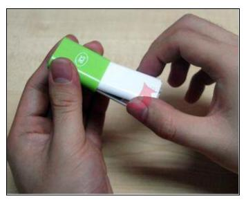
5. Remove the cover to reveal the SIM-sized card slot and Micro SD slot.
