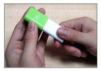
2. To close the cover of the USB connector, pull up the green cap.
