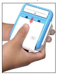
3. Remove the cover completely to reveal all three available SAM slots.
