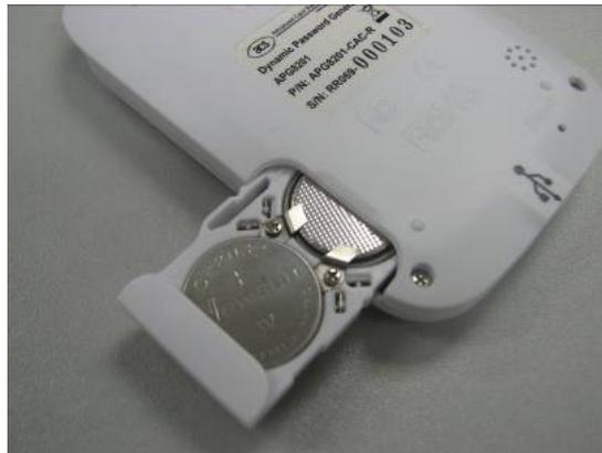
**Figure 5:** APG8201 with Battery Taken Out
