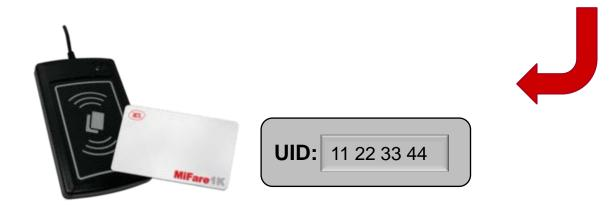
The reader detects the card and displays the Unique Identifier Number on the text entry box of any software application
