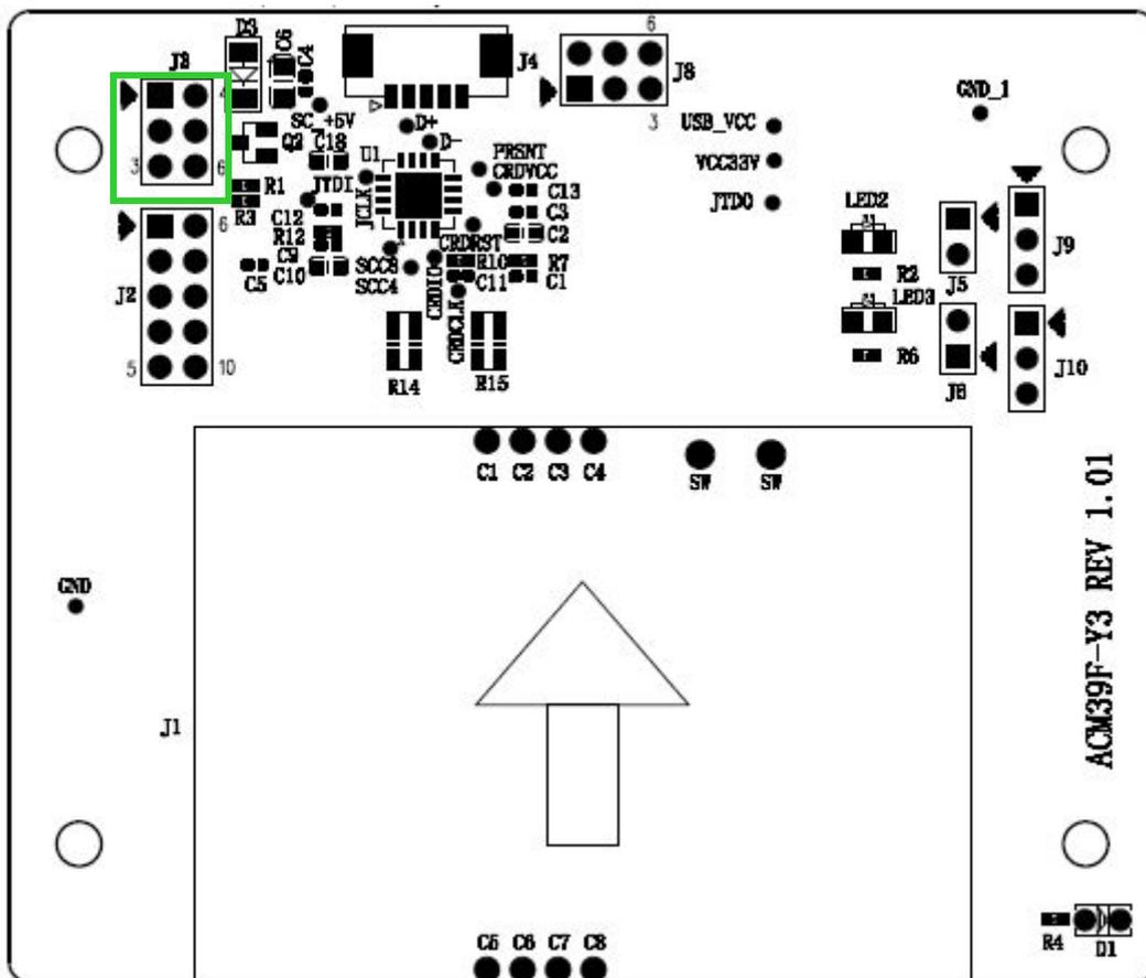
Figure 6: ACM39U-Y Card Detection Signal Configuration
