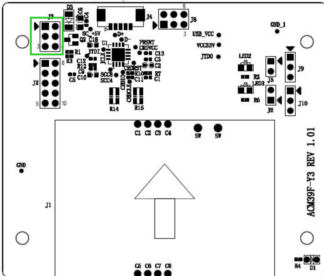
Figure 3: ACM39U-Y Card Detection Configuration
