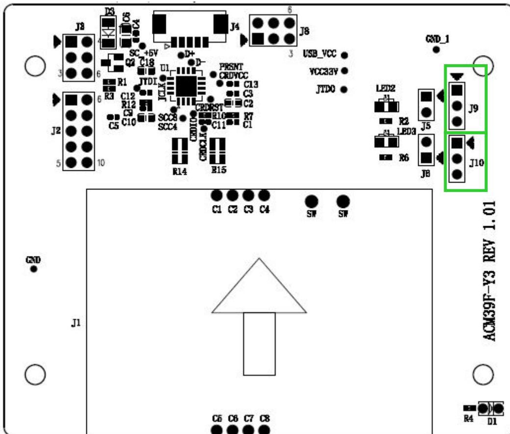
**Figure 9:** ACM39U-Y Extended Power and Card Operation Status Signals
