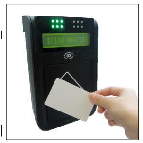
ACR300 Bus Validator is designed specifically for use in Automatic Fare Collection systems (AFC) for public transport.
