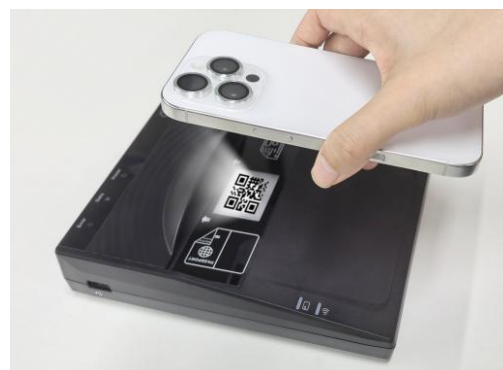
Figure 7: Scanning QR codes on a smartphone screen
