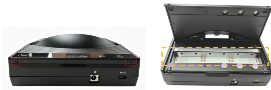
Figure 4: Half-enclosed light shield and OCR MRZ scanning glass window
