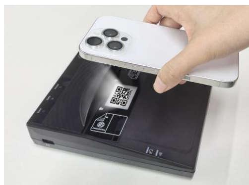
Figure 7: Scanning QR codes on a smartphone screen
